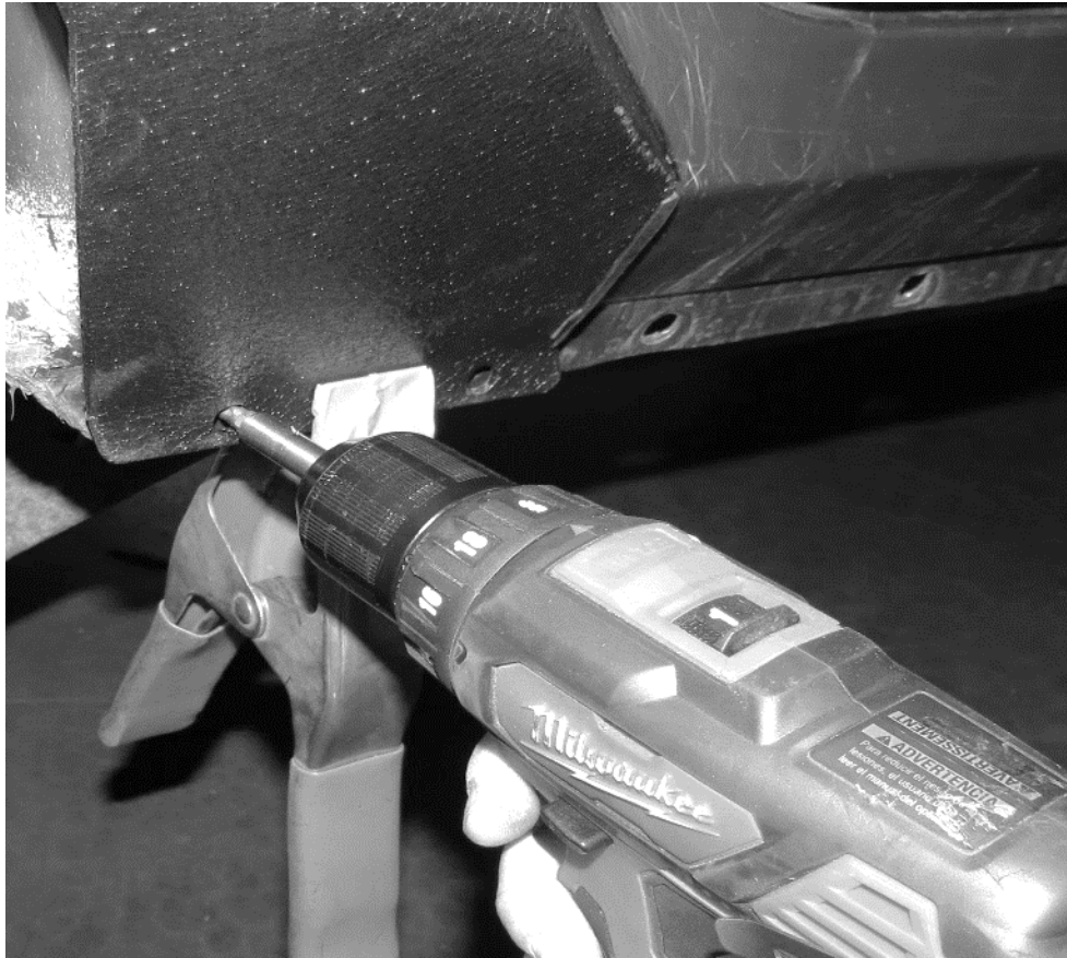
(Figure 11) Use 1/4" drill bit to drill out both holes in the pinch weld using fender as a guide.
