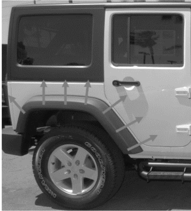
(Figure 6) Remove the factory fender flare by grabbing firmly and pulling radially out and away from the vehicle.
