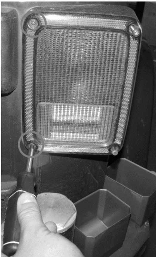
(Figure 3) Remove the 2 inside screws holding tail lights to the body.
