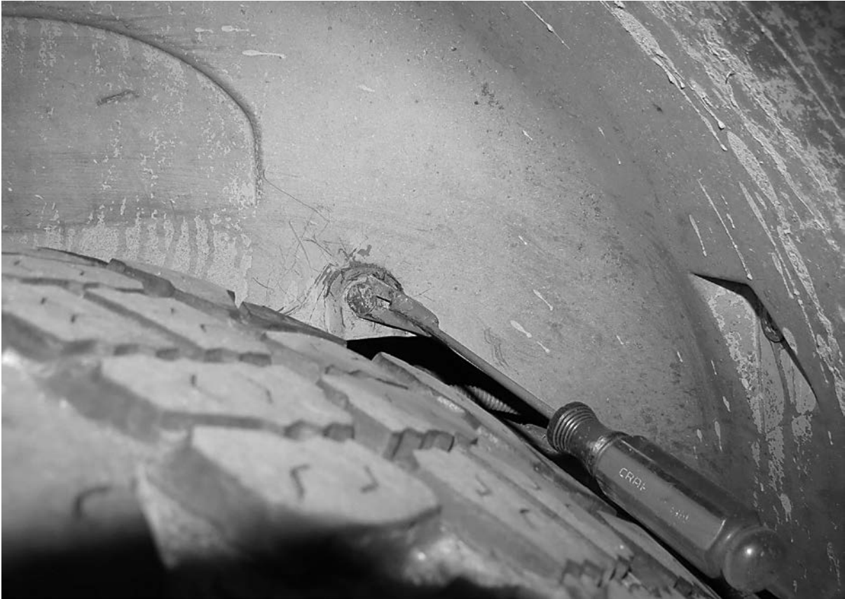
(Figure 4) Pry to remove the plastic fasteners that are securing the inner fender liner.
