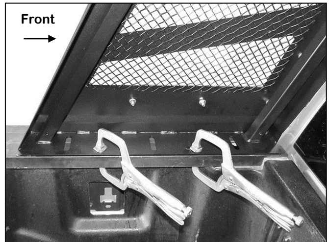
(Fig 6) Use clamps to temporarily hold Rack in position (Driver/left side illustrated)
